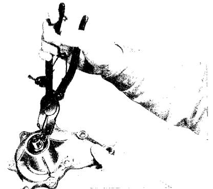
Fig. 3-9 Installing snap ring
