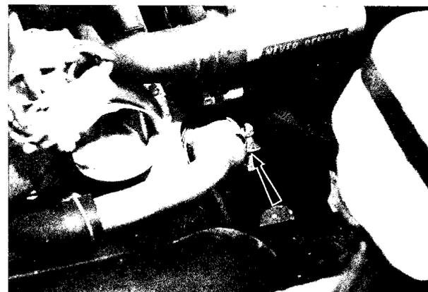
Fig. 1B-8 Removing air pipe
